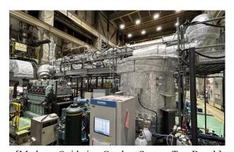
[Methane Oxidation Catalyst System Test Bench]
