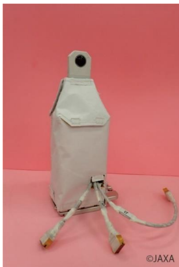
all-solid-state lithium-ion battery on-orbit experiment equipment (Space AS-LiB)
