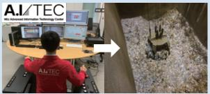
Remote operation of the waste crane from A.I/TEC.
