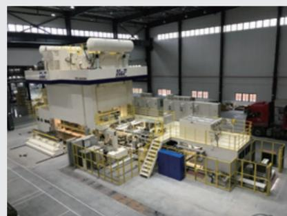
Press machines for automotive parts manufacturing in China (transfer press)
